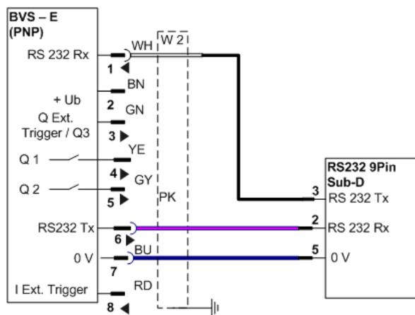
Fig. 9-1: Wiring the RS232 interface to a Sub-D 9-pin connector
