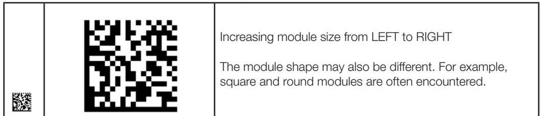
Using a high-quality printer **module sizes** of 0.2 mm can be printed. A DMC code with 12 x 12 bits has then an area requirement (including L- and Alternating Pattern) of 2.8 x 2.8 mm.
