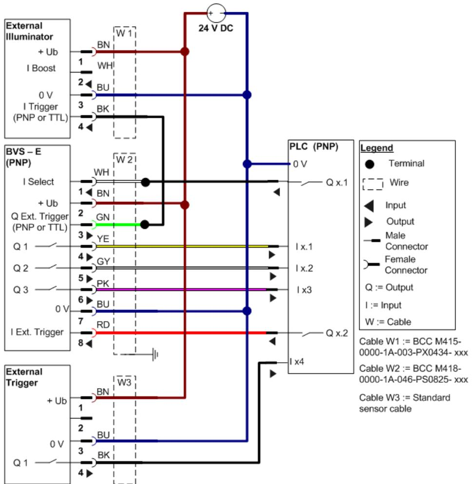
Fig. 3-6: Wiring diagram of the BVS-E sensor
