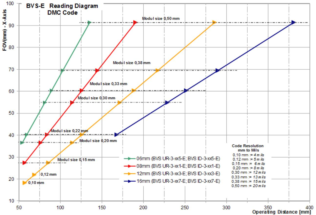
Fig. 16-7 Read field diagram for a Data Matrix code
