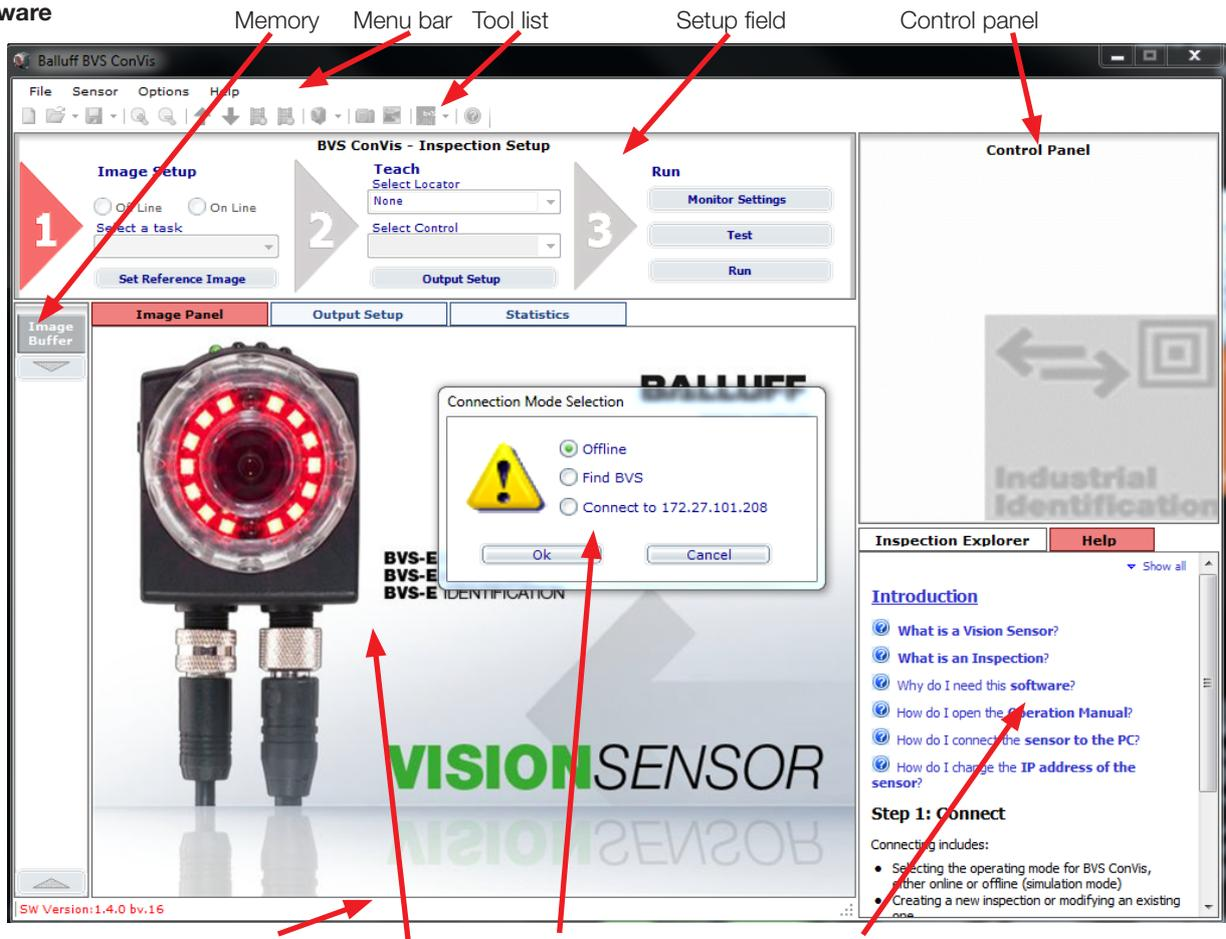
Fig. 12-1: BVS user interface - Overall view
