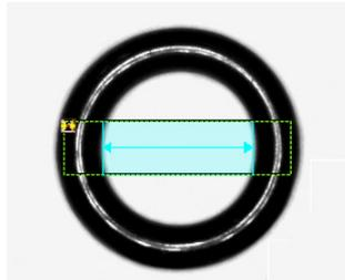
Fig.8-2a: O-Ring with correct size
