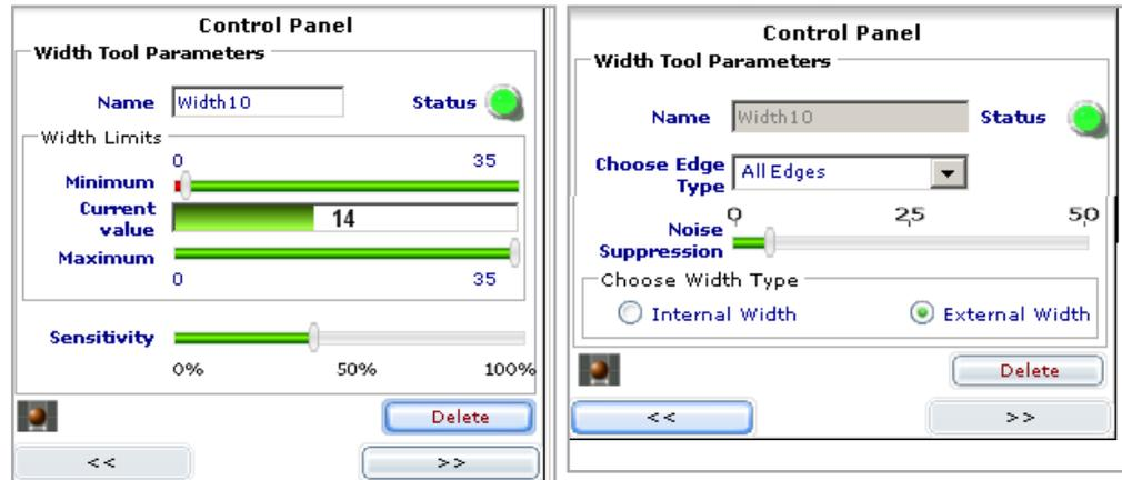
Fig.8-8: Control panel for Width, page 1 and page 2
