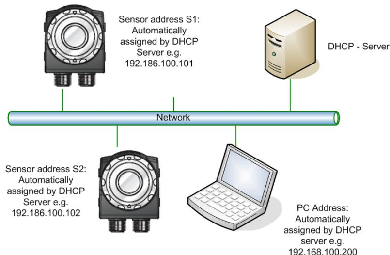
Fig. 12-2: DHCP connection of the sensor
