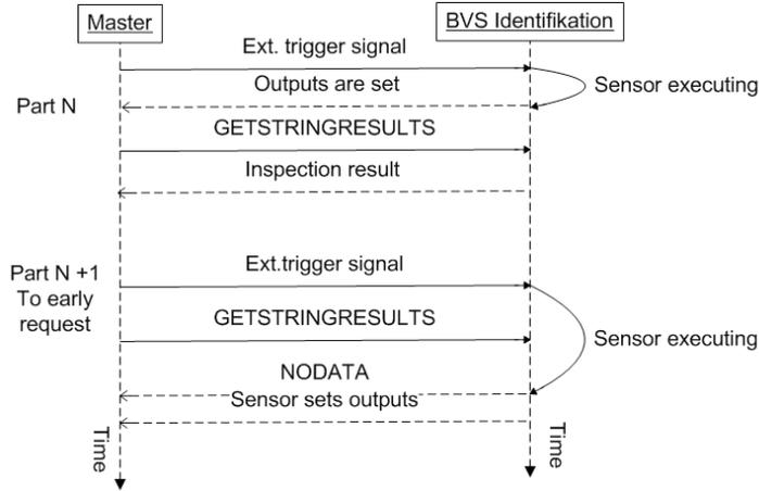
Fig. 9-2: Synchronous communication
