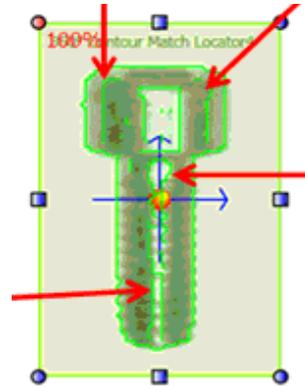
2.) Removing weak reflection contours using the Noise Suppression parameter. Contours with weak contrast or short length are removed by adjusting the Noise Suppression parameter.
