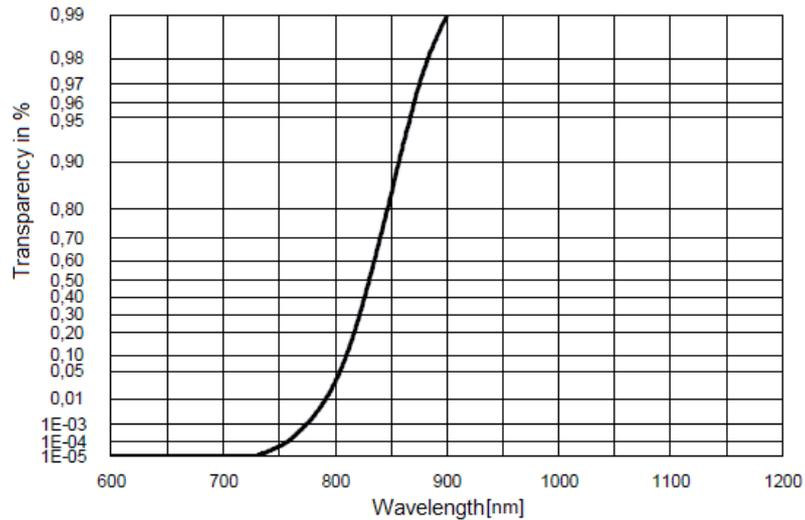
Fig. 16-3: Filter diagram of infrared models
