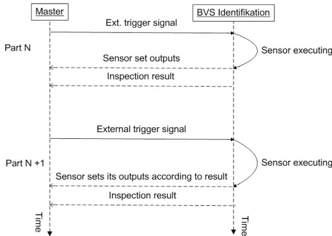
Fig. 9-3: Asynchronous communication
