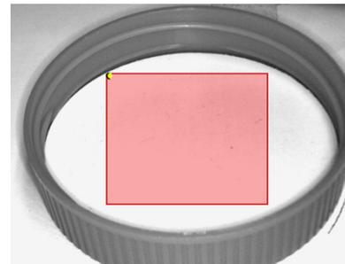
Fig. 8-1b Inspection for the correct printing NOK
