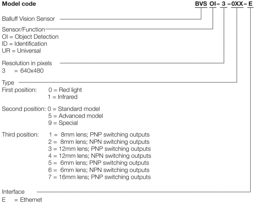
Each sensor is marked on the back side with the model and ordering code as well as the serial number:
