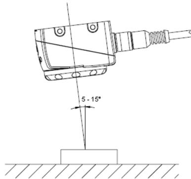
If you want to inspect an object having reflecting surfaces, we recommend installing the BVS at an angle of 5 to 15 degrees to the vertical axis to prevent unwanted reflections.
