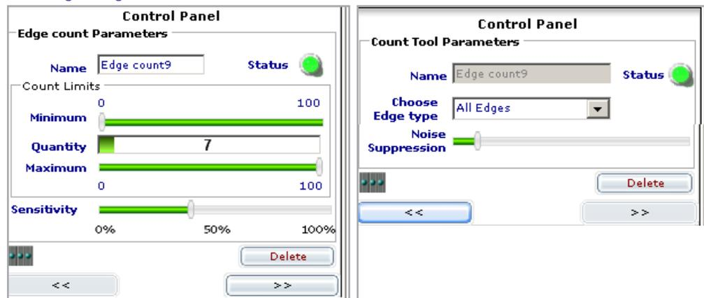
Fig.8-7: Control panel for “Count edges” page 1 and page 2
