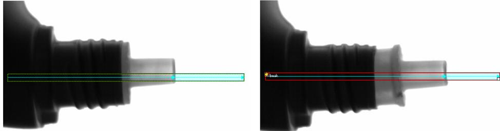
Fig. 8-4a Position checking of the spout of a dish liquid bottle: **OK**
