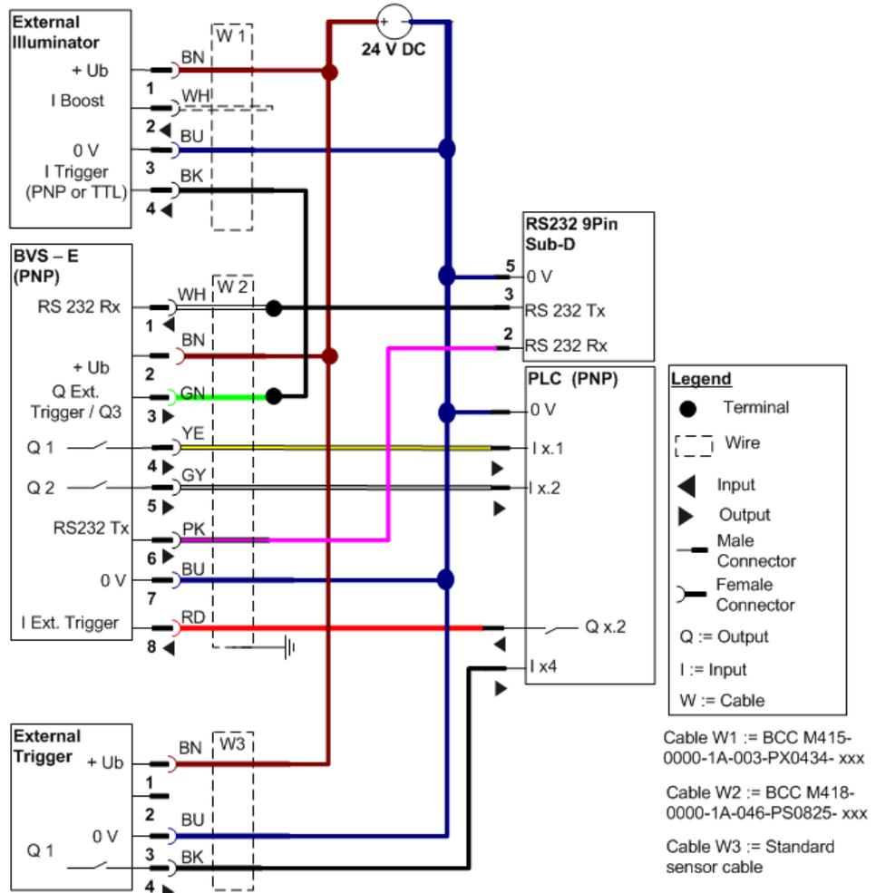
Fig. 3-7: Wiring diagram of the BVS-E sensor ID and UR
