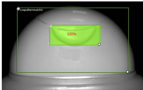
Fig. 8-3a Pattern detection of a shampoo bottle seal:
