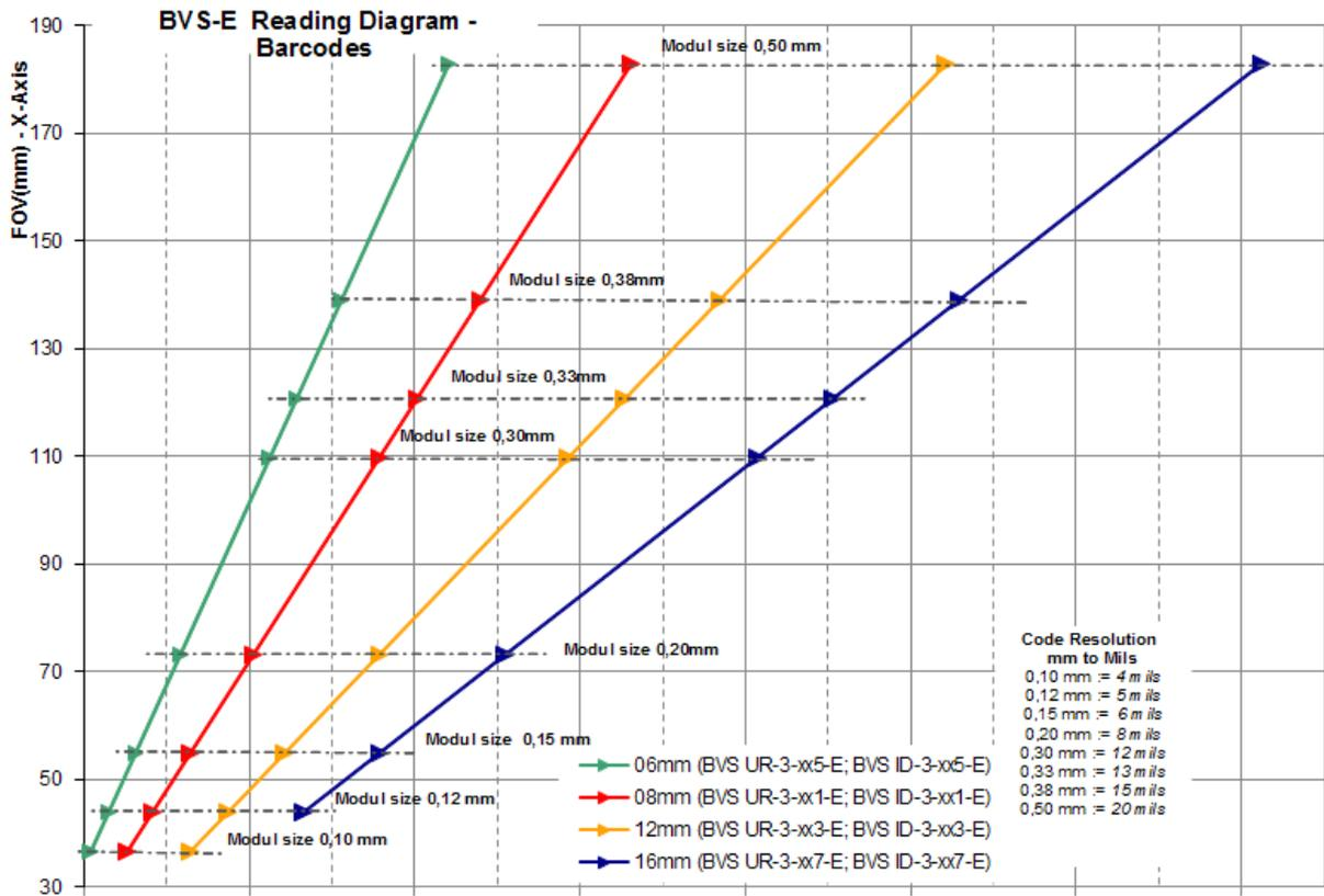
Fig. 16-6 Read field diagram for a barcode
