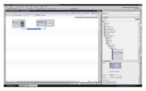
The module BNIPNTxxx105Z015 with the submodules PN-IO, port 1-M12, port 2-M12 are used for Profinet communication.
