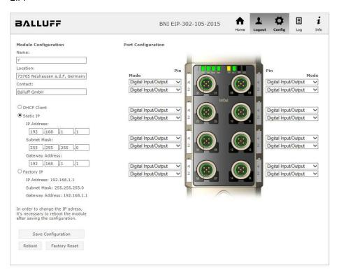
The parameter set "Module Configuration" on the left side is used by clicking "Save Configuration" and permanently stored in the device.
