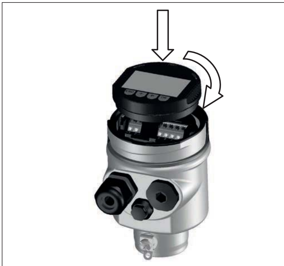
Fig. 17: Insertion of the display and adjustment module with single chamber housing
