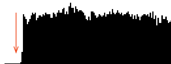
Fig. 3-7: Light band incorrectly aligned, left edge of the CCD not illuminated
