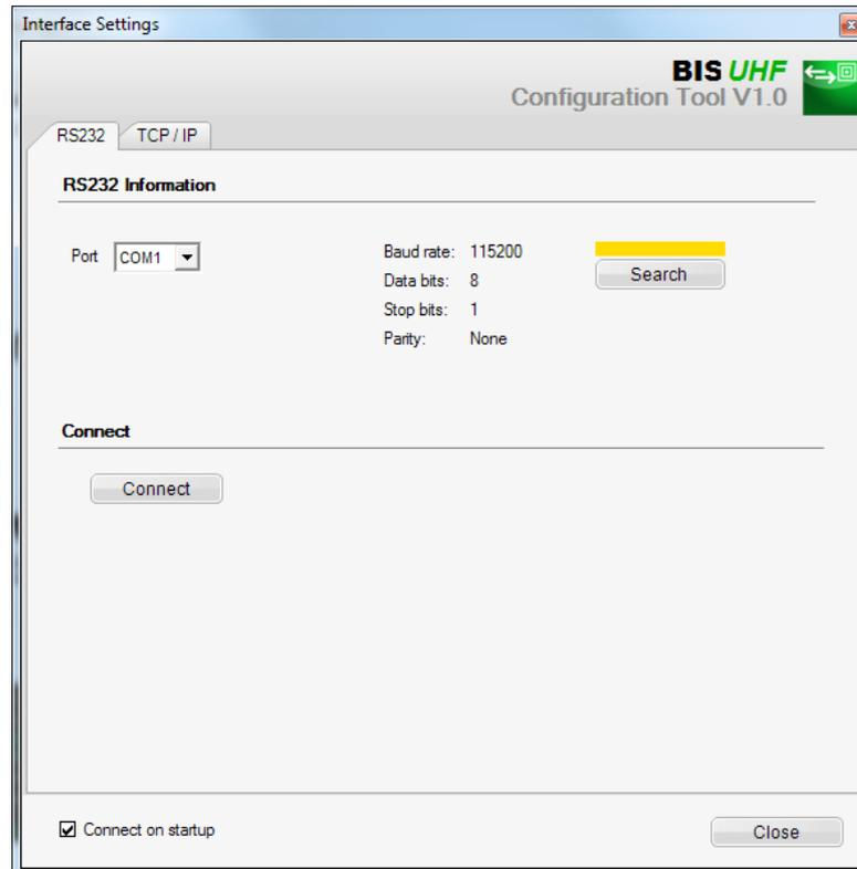
When the program starts, the device automatically connects if "Connect on startup" was selected in the "Interface Settings" window (factory setting).
