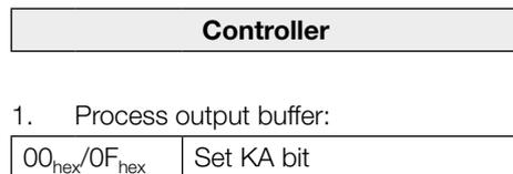
The antennas are switched back on by resetting the KA bit.
