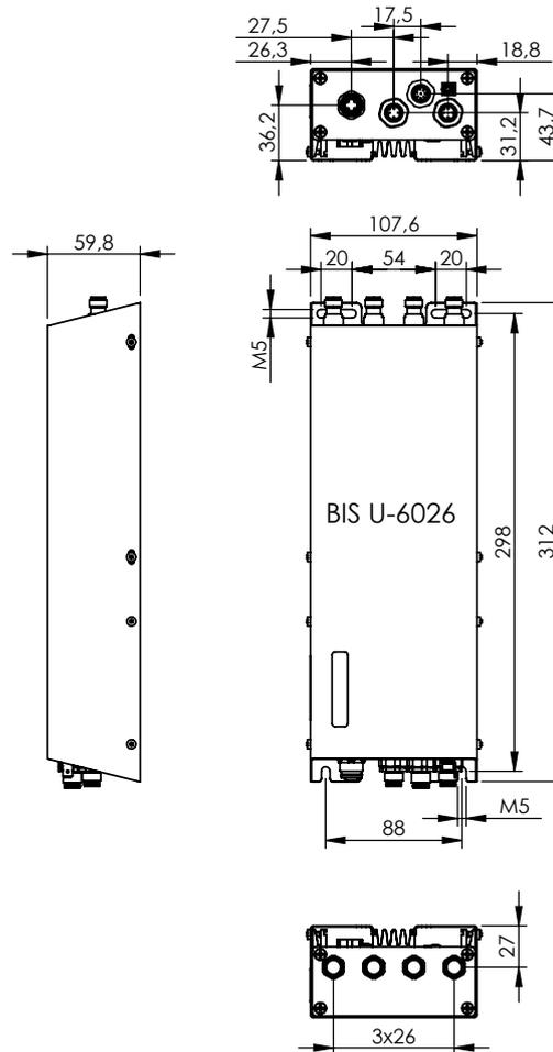
Figure 4: Dimensions of the BIS U-6026-...-ST35 (in mm)
