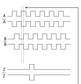
90° phase shift between A and B — In this example, B lags A by 90°, indicating FORWARD position change
