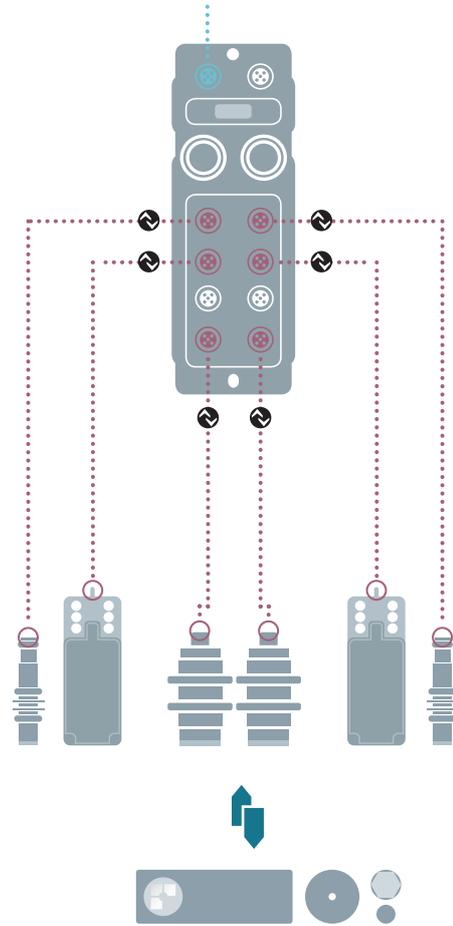
**IO-Link network block as the processor unit**
