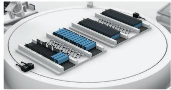
RELIABLY CHECKING POSITIONS USING INDUCTIVE FACTOR 1 SENSORS
