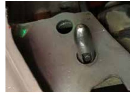
PHOTOELECTRIC FALSE NUT PRESENCE
