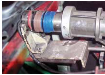
BROKEN OR WORN OUT SLIP RINGS
