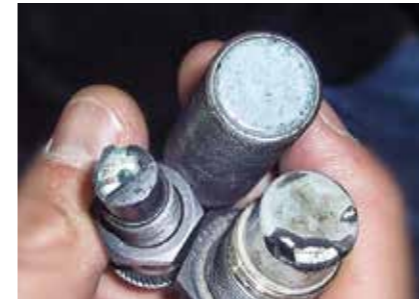
SENSOR FACE DAMAGED BY IMPACT
