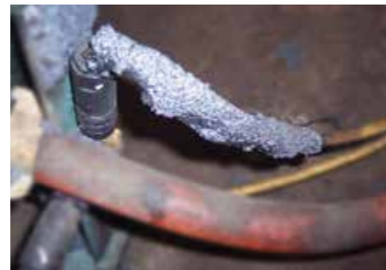
SENSOR CABLE BURN-THROUGH
