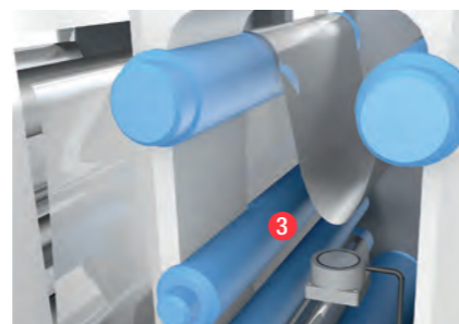
SHEET FEEDING FOR THE COIL BUS ultrasonic sensors
