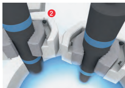
ASSURING THE CORRECT ELECTRODE POSITION BES inductive sensors
