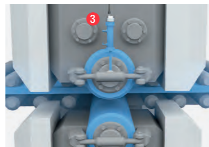
3 SETTING THE ROLL GAP PRECISELY BTL magnetostrictive sensors
