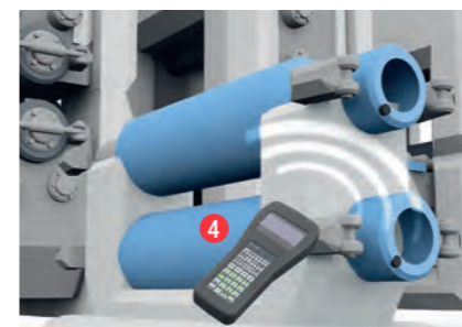
4 QUALITY ASSURANCE AT THE ROLLING STAND BIS industrial RFID systems
