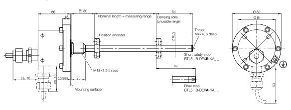
Model J, flange Ø 18 mm, pitch circle Ø 76.2 mm, Cable outlet radial
