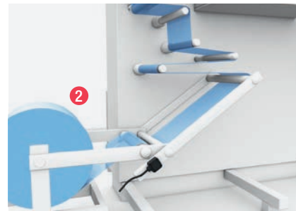
ROLL GUIDING BSI Inclination Sensors
