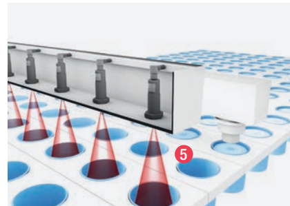
CHECKING THE PRESENCE OF THE CONTAINER FOR SECURE FILLING BUS Ultrasonic Sensors
