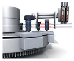
If very small parts need to be reliably detected and if tight installation conditions leave no space for even a mini sensor, fiber optics are the choice.
