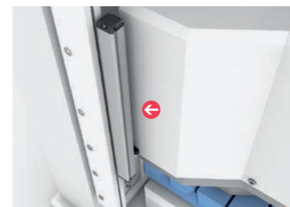
CONTINUOUS MEASUREMENT OF NOTCHING TOOL POSITION BTL magnetostrictive sensors
