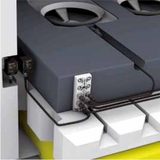
The inductive coupling system serves as a contact-free connection between the press and the tool. Typically the base is mounted in the bolster of the press in a common area.
