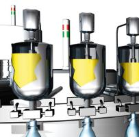
Precision dispensing and sanitary filling applications require precision performance and purpose-designed features. The Micropulse SF sanitary fill sensor is constructed from high-grade stainless steel and conforms to 3-A Sanitary Standards.
