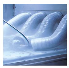
Design and build a prototype, abuse it until it fails, analyze the failure, improve the design, test it again. That's what Highly-Accelerated Life Time (HALT) Testing is all about. In-house HALT testing assures that potential design weaknesses are identified and subsequently eliminated.
