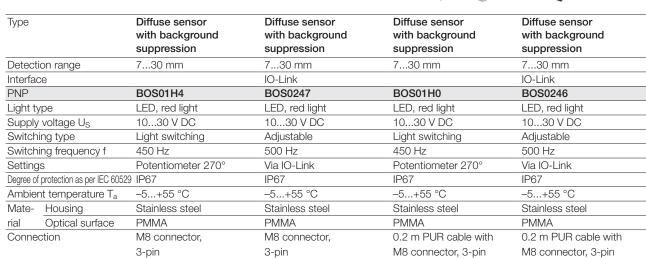
IO-Link functions: operating distance and hysteresis adjustable, switching type and switching modes selectable, diagnostic functions
